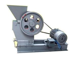
pressure on the coarser material while also permitting the finished material to pass through the jaws. A hopper is provided at the top for feeding material. The smooth jaws ensure a uniform product.
